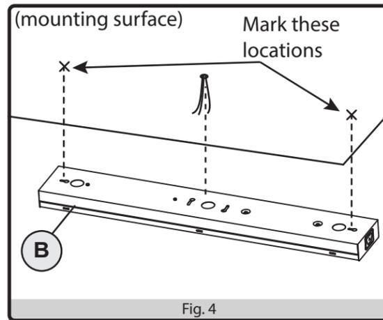
5. **DRYWALL MOUNTING:** If the mounting holes go through drywall without a stud, drill four small pilot holes using a 1/8-in. drill bit (not included), and install drywall anchors (BB) into the holes with a hammer (not included).
