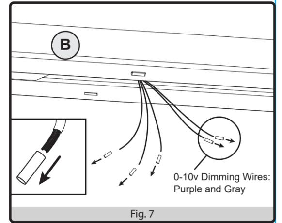
8. Connect the fixture wires to the supply wires -- black to black, white to white, and green to copper/bare. **WARNING:** If there is no ground supply wire, stop installation and consult a qualified electrician.
