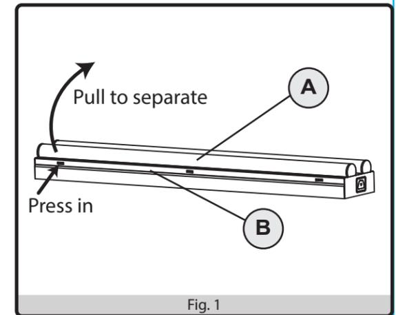
2. Locate the wiring quick disconnect connectors between the two halves and release the connectors to separate the wires between the two halves. Set aside the LED cover assembly (A).
