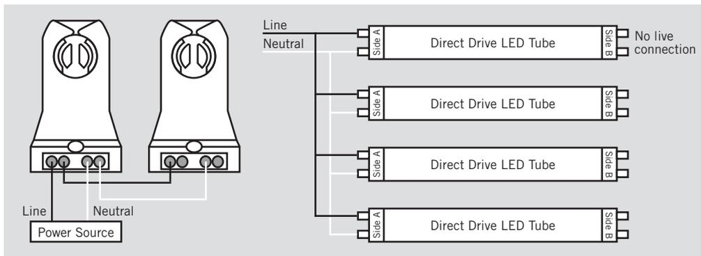
For Single-ended wiring, do not install product in a fixture with shunted lampholders (found in all fixtures using instant start ballasts). If the current lampholders are shunted, remove them and replace them with non-shunted lampholders. Make new connections directly to terminals as indicated above. Keystone can provide any style replacement lampholders. Call us at 800-464-2680.
