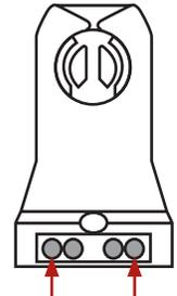
Connect wires directly to these terminals
