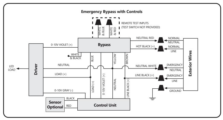
**EMERGENCY BYPASS OPTION:** Connect the BLACK and RED wires from the fixture to the normal, non-emergency AC wires to detect whether or not the fixture is in emergency mode.
