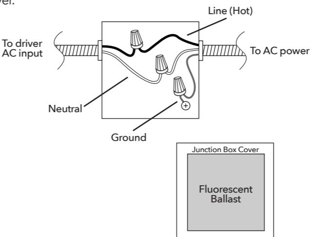
**IMPORTANT:** The fluorescent ballast must remain attached to the junction box cover.
