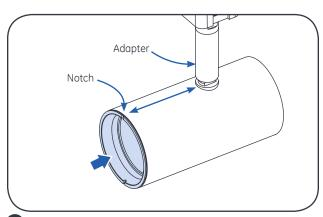
4 Install the new lens: Align notch with the adapter.
