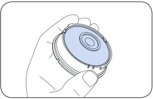
3 Inspect field changeable lens to ensure no dust particles are trapped inside.
