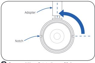
Remove old lens: Rotate the cap 90 degrees counter-clockwise until the notches fully align with the adapter and pull out.
