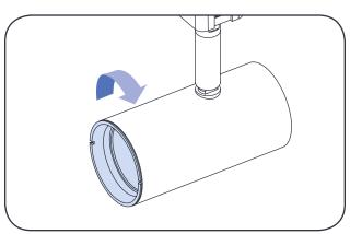
**5** Rotate lens 90 degrees clockwise to lock it in place.
