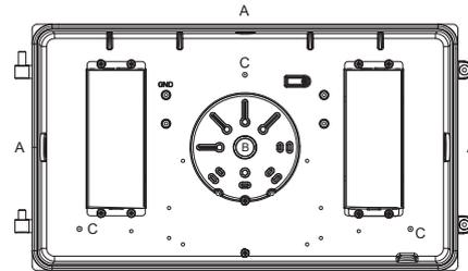
A - 1/2" NPS tapped holes (surface conduit or photo control)
