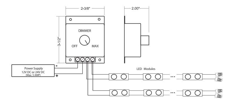
\*Allanson LED Dimmer (PWM) will dim all 12V and 24V LED Modules, except for the 1 Watt (ACLW-CW-1W) and 3 Watt (ACLW-CW-3W) modules, and the LED Saber.
