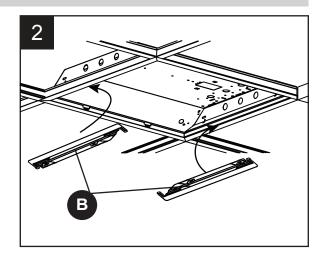
3. Using the sheet metal screws (C) provided, drill through the existing housing and secure the two brackets (B) on each side with two screws each with the tabs on each of the brackets (B) as shown.
