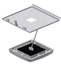
UNV Accessory Kit (673427) Includes mounting panel with auxiliary latch, 4 inner flange brackets and hardware to attach panel to fixture
