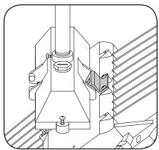
2 Lift fixture up and hang on pendant mount box using hinge piece.
