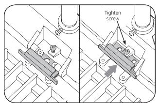
4 Swing fixture closed and secure with the slide clip. Lock slide clip in place with screw.
