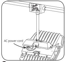
Feed the AC power cord through the conduit and into the junction box.
