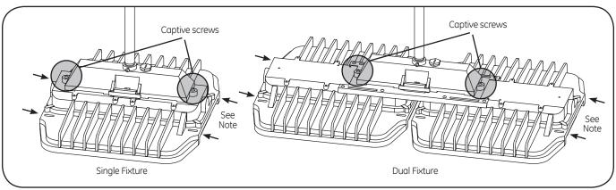
Secure pendant mount box to fixture by fully tightening the captive screws on the sides of the pendant mount box to the fixture.
