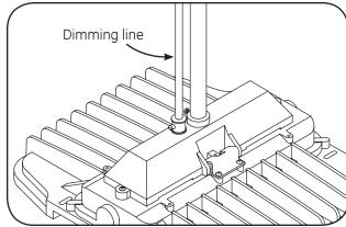
6 Dimming line can be run through 1/2" NPT conduit installed to the top of the mount box.
