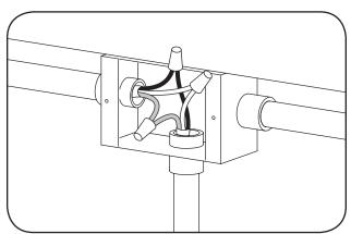
6 Connect the green (ground), black (line) and white (neutral) wires of the AC line to the similarly colored wires of the fixture's power cord using UL listed wire connectors. Close junction box.
