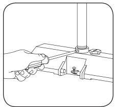
Attach pendant mount box to 3/4" NPT conduit. Determine rotation of fixture and lock orientation in place with provided set screw.
